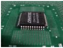
Chip legs are in the grooves, thus touching the pads and holding the chip in place
